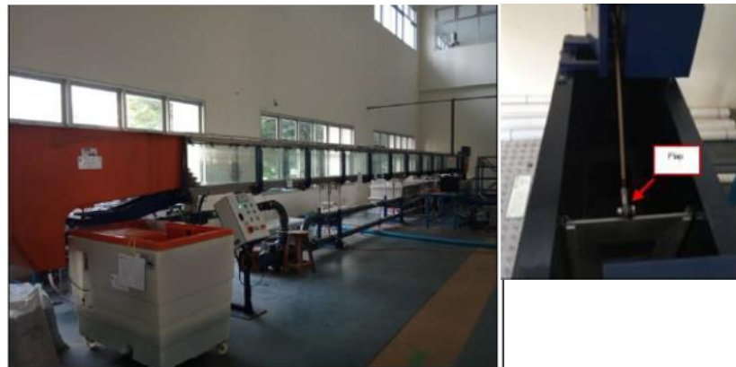
FIGURE 3. Wave flume and wave generator flap-type used in this study
